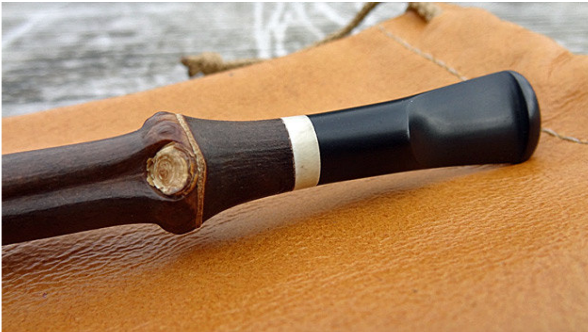
Figure 1 Notice the tight tolerances and smooth lines between the intersecting parts of the shank (made of bamboo), the accent ring (made of bone), and the bit (made of ebonite).
