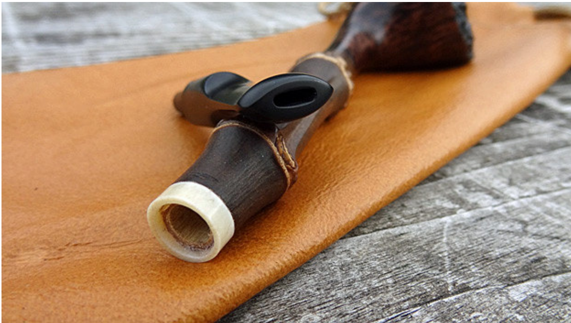
Figure 6 A clear look at the deer bone accent ring that melds the bamboo shank to the ebonite stem.
