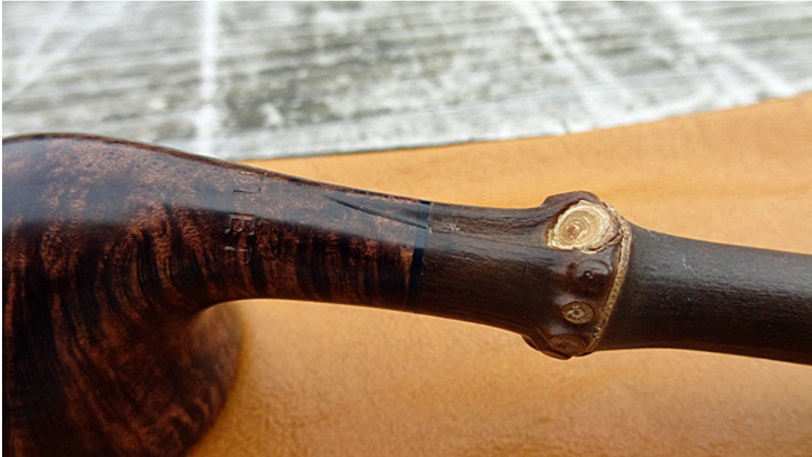
Figure 3 Notice the smoothness and flow between the bamboo, black acrylic accent washer and the stummel. Also, take a look at how precise the forming is on the briar in order to make the contours of the bamboo flow into the pipe itself.
